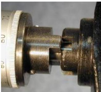
**Disengaging the handwheel**
